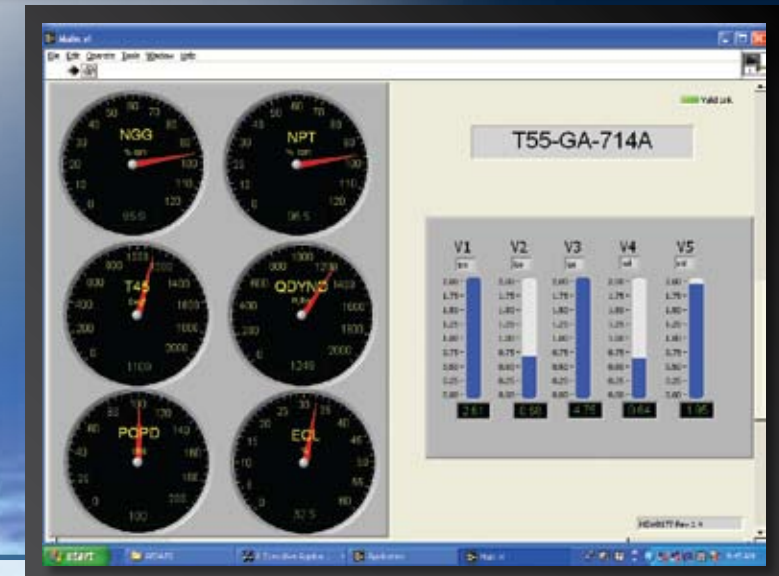
Pictured at left: On the upper half of the screen, the grid window displays up to 32 parameters outlining the parameter name, the value of the parameter and measurement units. The lower right screen displays the bar graph/round dial window, providing visual verification that testing is within range of a given condition.
